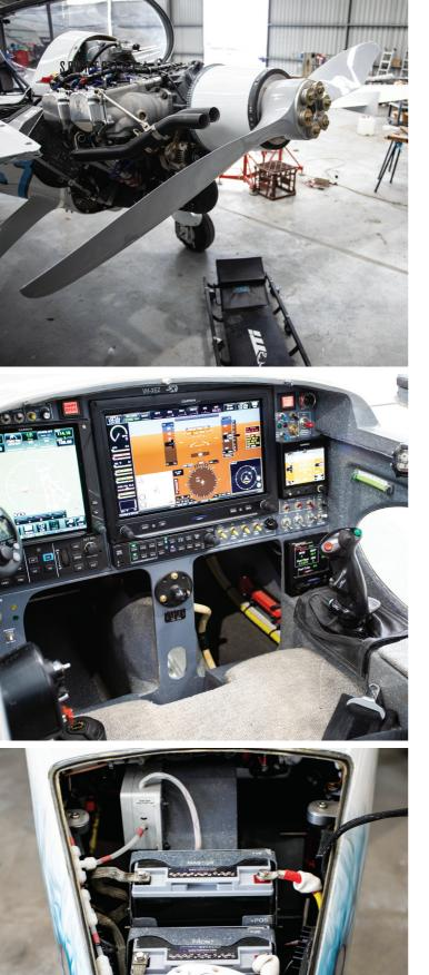
For example, one of the toggles on the joystick controls the direction of a large LED Headlight installed in the nose of the plane for taxiing and better vision at night.
